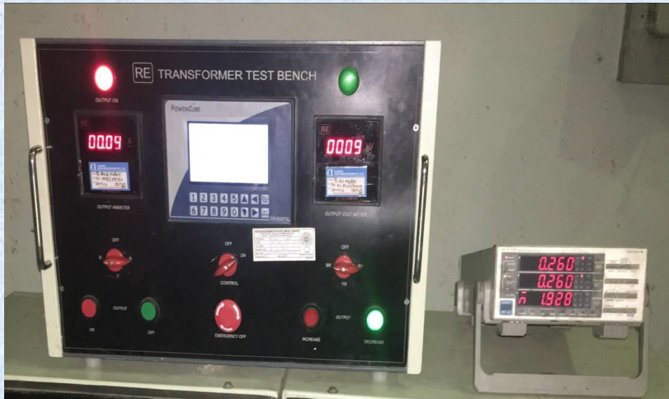
3-Phase Transformer Test Bench, 75 kVA, 2000 V & 52 Amps
